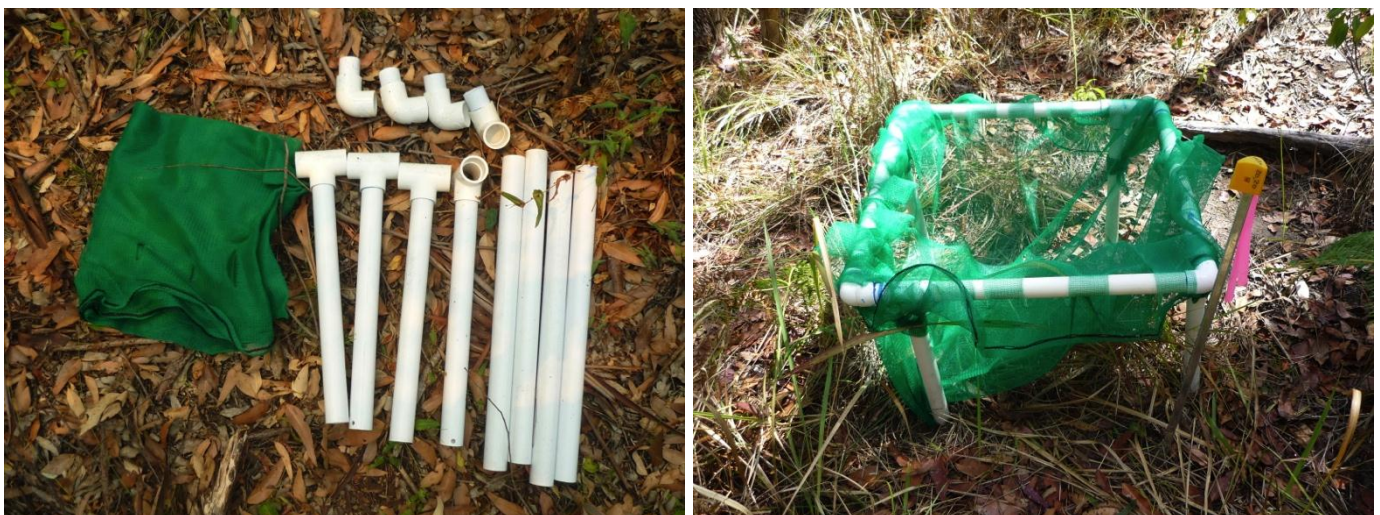
Figure 33: Photographs showing litterfall trap materials (L) and an assembled litterfall trap (R)
